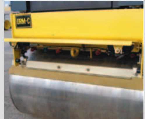
Wind protected, quick-disconnect spray nozzles with dual scrapers per drum.
