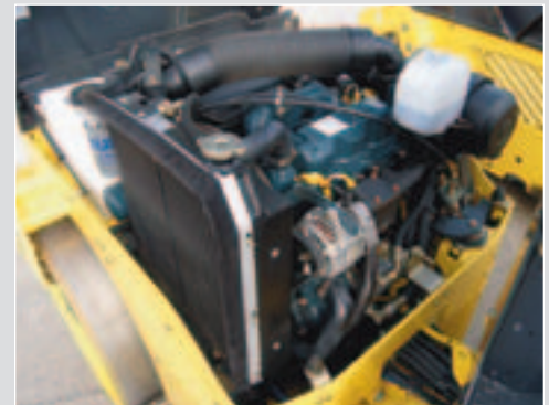
Easy access to engine and drive components for simplified servicing
